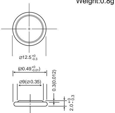
**Note:** This bare cell diagram is for size reference only. Please refer to the tab configurations at the end of this section for available tabs.
