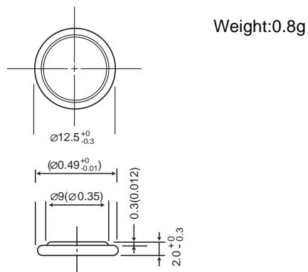
**Note:** This bare cell diagram is for size reference only. Please refer to the tab configurations at the end of this section for available tabs.
