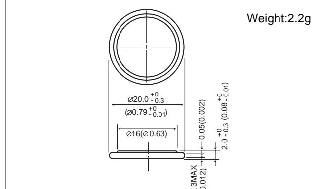
**Note:** This bare cell diagram is for size reference only. Please refer to the tab configurations at the end of this section for available tabs.
