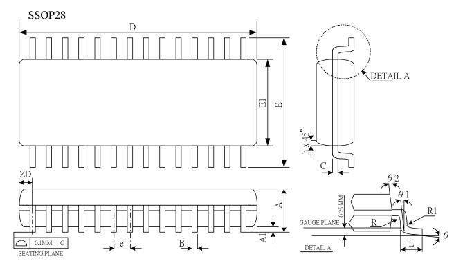
NOTES: DIMENSION D DOES NOT INCLUDE MODE PROTRUSIONS OR GATE BURRS. MOLD PROTRUSIONS AND GATE BURRS SHALL NOT EXCEED 0.006 INCH PER SIDE
