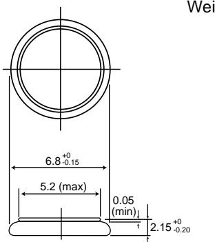
**Note:** This bare cell diagram is for size reference only. Please refer to the tab configurations at the end of this section for available tabs.
