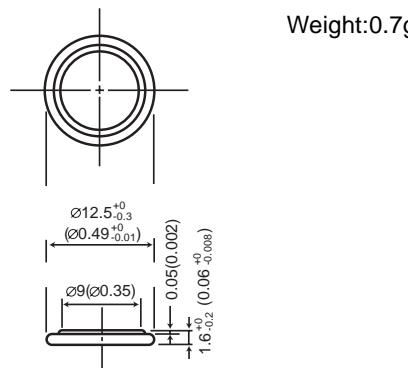
**Note:** This bare cell diagram is for size reference only. Please refer to the tab configurations at the end of this section for available tabs.
