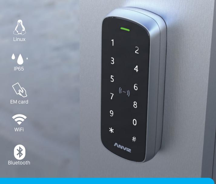
M3 Pro is a metal casing, IP65 water-proof design compact access control device, suitable for outdoor applications. It supports 13.56MHZ mifare card and 125KHZ EM card dual frequency module. The touch backlit keypad, support TCP/IP and RS485 communication convenient for customers to use. The M3 Pro has both built-in relay for direct lock and standard wiegand output, which can be work as standalone access controller and RFID reader.
