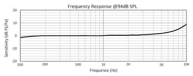
Typical frequency response curve relative to the sensitivity at a frequency of 1 kHz
