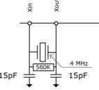
The programmable delay guarantees that the oscillator has settled before the measurement starts. For ceramic resonators  $480 \ \mu s$  will be sufficient. By this measure the average current consumption can be drastically reduced. Example:
