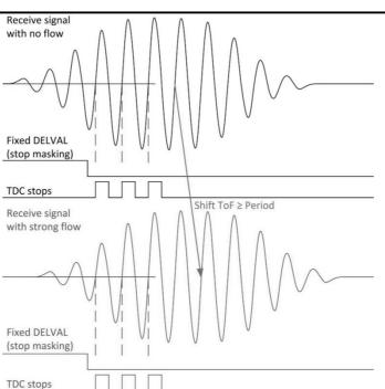
There is still another source of getting wrong measurements. Dirt deposition on the transducers, spool piece mirrors and housing will lead to signal damping e.g. from  $\pm 400$  mV to  $< \pm 80$  mV. The figure below shows how this will affect the first wave detection at a given, fixed offset for the first wave detection. Once the first wave amplitude is below the offset level the measurement result will jump by one period.
