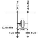
The settling time of this oscillator is about 3 s after power-up. The 32.768 kHz oscillator cannot be switched off.
