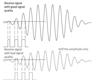
With the SSP1922's first wave detection the time-of-flight measurement is related to the first wave and gets independent from temperature and flow. Miscalculations due to wrong zero crossing assignment are no longer possible.
