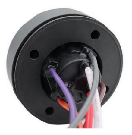
The entire RCT-240 series twist-lock receptacles were designed for the lanterns those intended to have an ANSI C136.10 -2006 receptacle to fit a twist-lock photocontrol. This series conform newly published ANSI C136.41-2013 to allow a LED lamp multi-controlled through the receptacle, and obtained cRUus certificates under UL file E188110.
