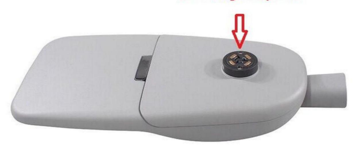
Disconnect power; wire the receptacle according to the diagram below. An arrow indicating NORTH on the top of the receptacle is used to assist correct direction. Push the photocontrol on and turn it clockwise to lock into the receptacle. Adjust the receptacle position if necessary.
