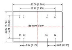
Note: Unit:mm[inch] Pin diameter tolerances :±0.10[±0.004] General tolerances:±0.50[±0.020]
