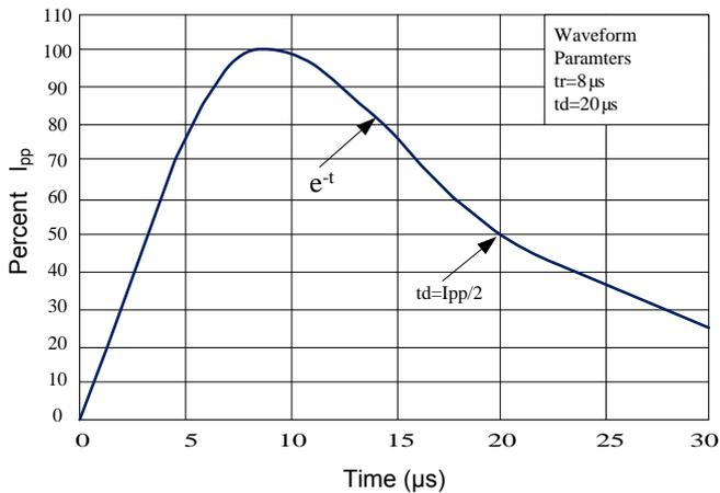
Figure 6: ESD Clamping( 8kV Contact per IEC 61000-4-2)
