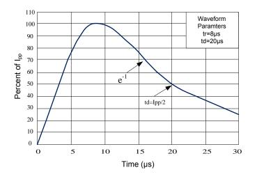
Figure 4: ESD Pulse Waveform (IEC 61000-4-2)
