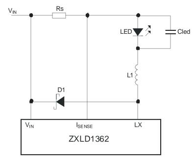
A value of 1µF will reduce the supply ripple current by a factor three (approx.). Proportionally lower ripple can be achieved with higher capacitor values. Note that the capacitor will not affect operating frequency or efficiency, but it will increase start-up delay, by reducing the rate of rise of LED voltage.
