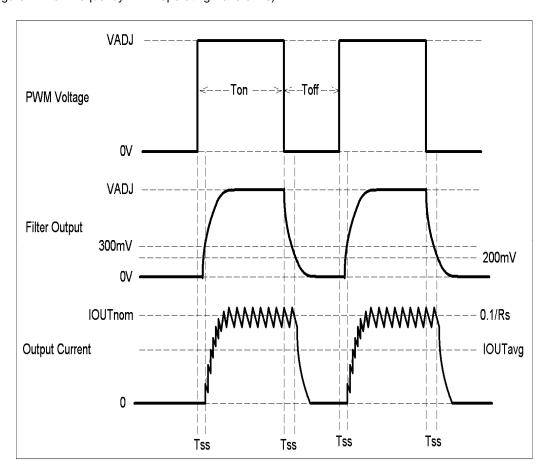
Figure 4. Low Frequency PWM Operating Waveforms
