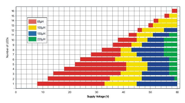
Figure 3. ZXLD1362 Minimum Recommended Inductor
