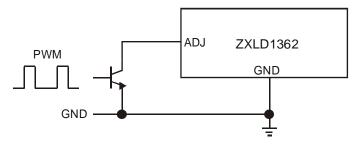
This scheme uses the 50k resistor between the ADJ pin and the internal voltage reference as a pull-up resistor for the external transistor.
