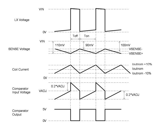
**Figure 2. Theoretical Operating Waveforms**
