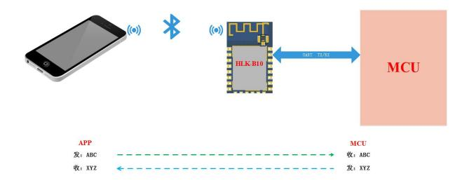
When the mobile phone APP and the module establish the Bluetooth connection, the data sent in the mobile phone APP is forwarded to the serial port of the module as it is, and the data sent to the module serial port will be forwarded to the mobile phone APP as it is.
