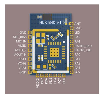
Figure 5 Schematic diagram of pin location
