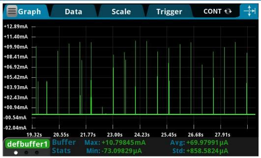
Figure 8 Working current graph when low-power sleep mode is enabled
