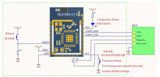
Figure 7 Basic minimum circuit (Enable low-power sleep function)
