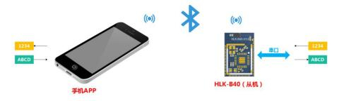
Figure 1 Schematic diagram of one-to-one Bluetooth connection transparent transmission function
