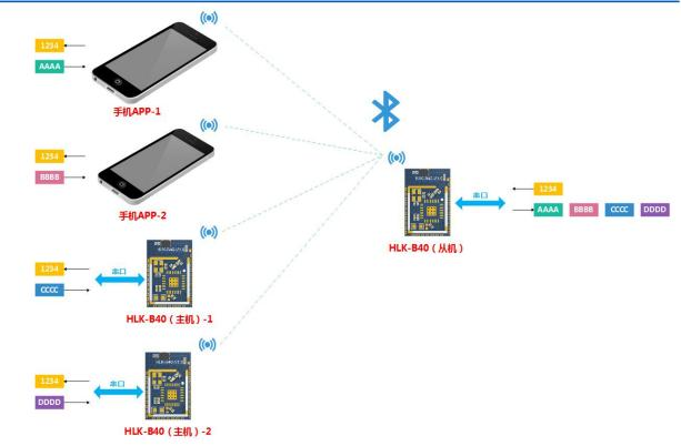
Figure 2 Schematic diagram of many-to-one Bluetooth connection transparent transmission function
