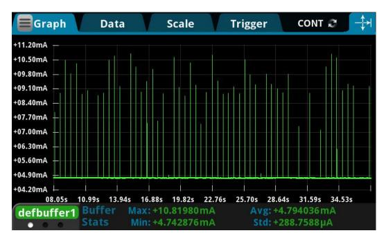
Figure 9 Diagram of working current when low-power sleep mode is disabled
