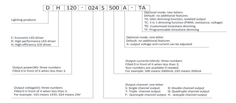
For example: DH120-024S500A-TA means: high efficiency LED driver; output power 120W; output voltage 24Vdc; output current 5000mA; single output; output voltage and current can be adjusted; with DALI dimming function and isolated output.
