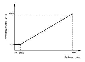
b. 0-10V dimming function for output current adjustment (Typical)
