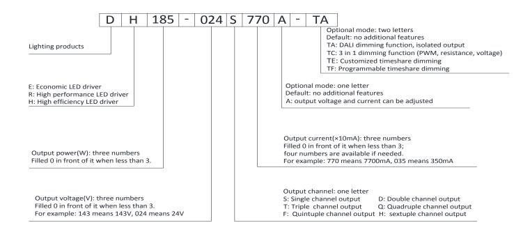
For example: DH185-024S770A-TA means: high efficiency LED driver; output power 185W; output voltage 24Vdc; output current 7700mA; single output; output voltage and current can be adjusted; with DALI dimming function and isolated output.
