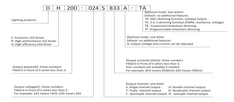
For example: DH200-024S833A-TA means: high efficiency LED driver; output power 200W; output voltage 24Vdc; output current 8330mA; single output; output voltage and current can be adjusted; with DALI dimming function and isolated output.
