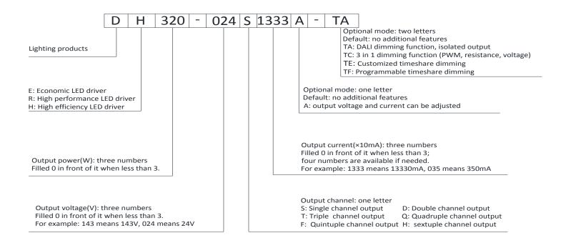
For example: DH320-024S1333A-TA means: high efficiency LED driver; output power 320W; output voltage 24Vdc; output current 13330mA; single output; output voltage and current can be adjusted; with DALI dimming function and isolated output.
