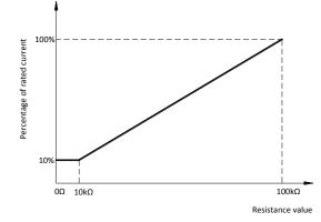
b. 0-10V dimming function for output current adjustment (Typical)
