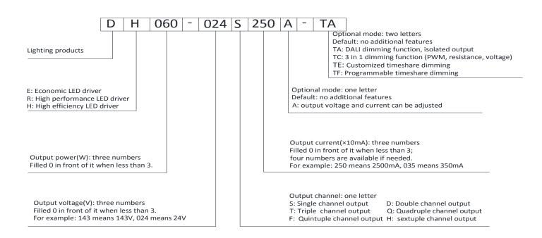
For example: DH060-024S250A-TA means: high efficiency LED driver; output power 60W; output voltage 24Vdc; output current 2500mA; single output; output voltage and current can be adjusted; with DALI dimming function and isolated output.
