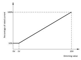
c. 10V PWM signal for output current adjustment (Typical): Frequency range: 200Hz~1.5KHz
