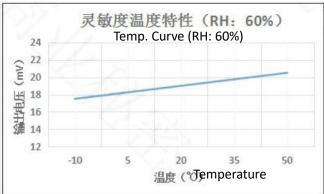
Fig5.Zero point at different temp.
