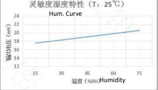
Fig7.Zero point at different humidity
