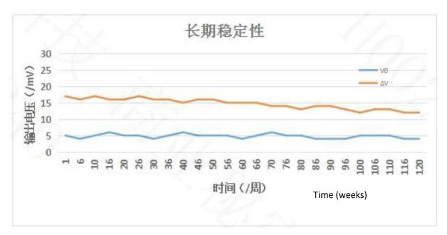
Fig11. Zero and Sensitivity stability curve
