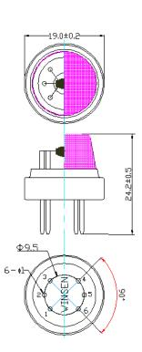
Fig1.Sensor Structure Unit: mm
