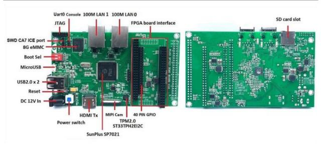
note : 40 PIN GPIO compitable Raspberry Pi
