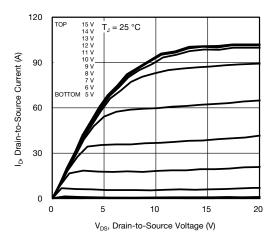
Fig. 1 - Typical Output Characteristics
