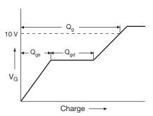
Fig. 18 - Basic Gate Charge Waveform
