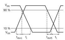
Fig. 15 - Switching Time Waveforms
