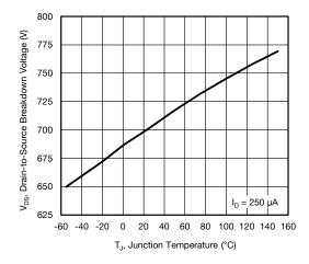
Fig. 11 - Temperature vs. Drain-to-Source Voltage
