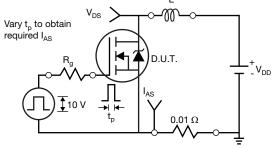
Fig. 16 - Unclamped Inductive Test Circuit
