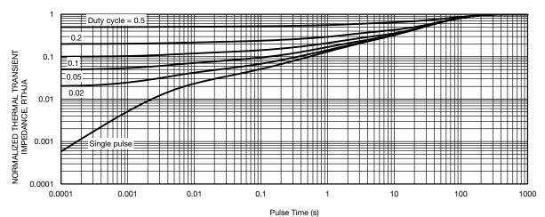
Fig. 13 - Normalized Thermal Transient Impedance, Junction-to-Ambient
