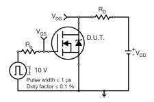
Fig. 14 - Switching Time Test Circuit
