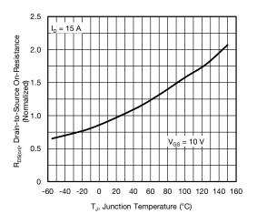
Fig. 4 - Normalized On-Resistance vs. Temperature
