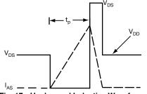
Fig. 17 - Unclamped Inductive Waveforms
