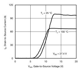
Fig. 3 - Typical Transfer Characteristics
