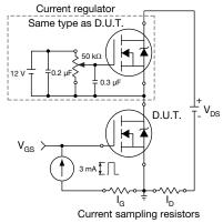
Fig. 19 - Gate Charge Test Circuit
