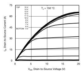
Fig. 2 - Typical Output Characteristics
