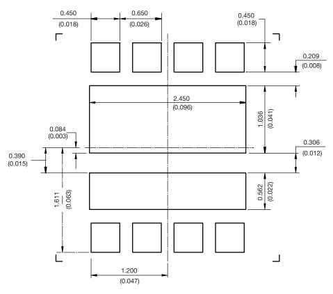
Recommended PAD for PowerPAIR 3 x 3 Dimensions in millimeters (inches) Keep-Out 3.5 mm x 3.5 mm for non terminating traces
