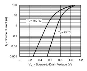
Source-Drain Diode Forward Voltage
