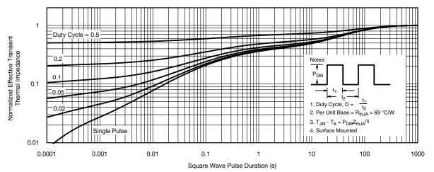
Normalized Thermal Transient Impedance, Junction-to-Ambient
