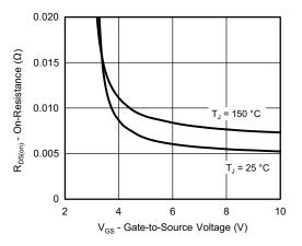
**On-Resistance vs. Gate-to-Source Voltage**
