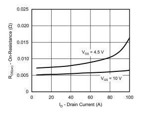
**On-Resistance vs. Drain Current and Gate**
