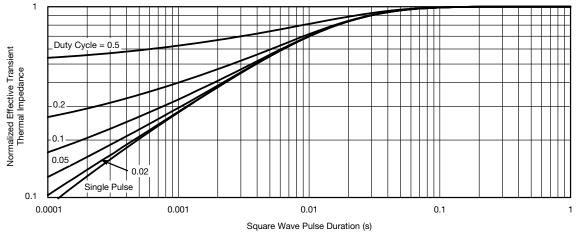
Normalized Thermal Transient Impedance, Junction-to-Case
